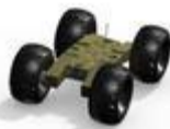
A computer rendering of the Vecna Robotics Porter UGV, which has now reached the early prototype stage. (Vecna Robotics)
